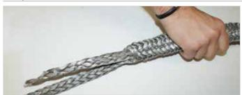
After both splice ends have been tapered, it is necessary that you smooth out the splice.
