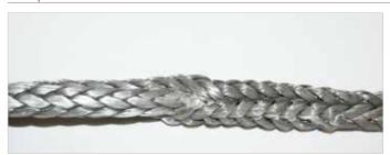
Into this opening, insert the rope end ...
