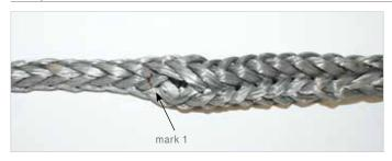
Use your finger or a splicing needle to make an opening at mark 1.
