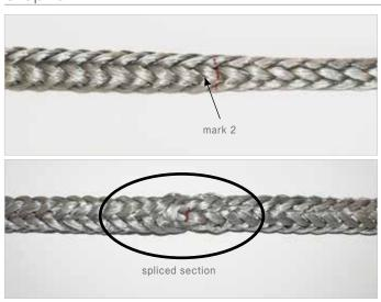
Once the splicing procedure has been completed, no rope end should be projecting at mark 2, on either side.
