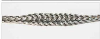
Push the rope together. This loosens it and makes the splicing procedure easier.
