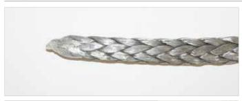
Use a knife to taper the two rope ends, and tape them with adhesive tape. In the case of hard ropes, the rope will also serve as splicing tool, while for soft ropes it may be necessary to use a splicing aid (splicing needle, see photo).
