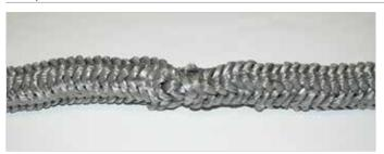
Now, push the splice together at the two rope ends.
