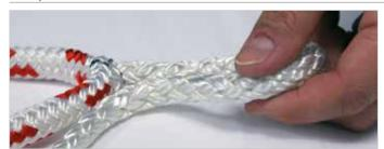
Now pull the core completely out of the cover.
