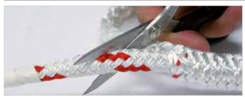
Cut off the cover obliquely about 15 cm from the point of transition and slip the core over the cover such that the cover disappears completely in the core.
