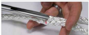
At mark 2, stick the splicing needle into the core and move it toward mark 3.
