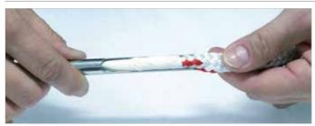
Insert the taped up tip of the cover into the splicing needle as shown on the left-hand side.
