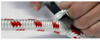
Pull the core toward the eye and cut it off very close to the exit point. Be sure to avoid damaging the cover when cutting off the core.
