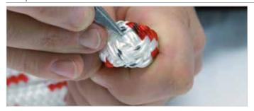
Bend the rope sharply at mark 2. Using an awl, open the rope's cover.
