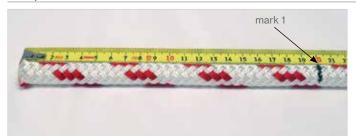
Mark the rope in a location 20 cm from the end of the rope (=mark 1)
