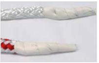
Make core and cover taper using sharp scissors ...
