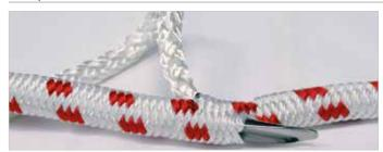
The splicing needle exits the braided cover 3 cm after the intersection (between cover and core). Pull the core through completely.
